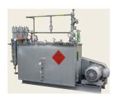
Compressor - A 3-stage compressor increases the acetylene pressure from .4 bars (6 psig) to 24 bars maximum (350 psig). Cooling coils and condensate traps are located at each stage, and the entire assembly of the compressor,
